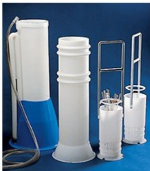
CONTENITORE PER PIPETTE H 503 MM PE/PP
